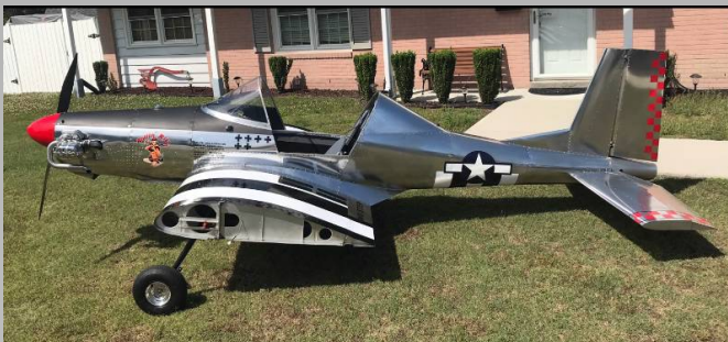
Wings are easily detached – undercarriage is attached to the center section which means fuselage remains on its wheels
